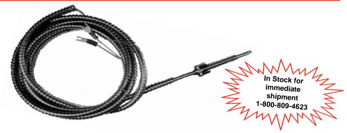
THE BAYONET Style Thermocouples are the most widely used thermocouple in the plastics industry. All styles are available in straight, 45° and 90° bend with flexible stainless steel leads. MOLDERS CHOICE offers all thermocouples in both TYPE J (iron - constantan) and TYPE K (chromel - alumel)
