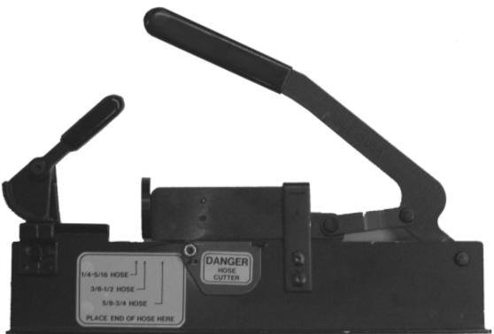
This unique tool combines a hose cutter with a toggle action that presses the fitting into hose, making every job easier, whether you are making one assembly or a hundred. It is designed to handle Push-Lok hose from 1/4" through 3/4".
